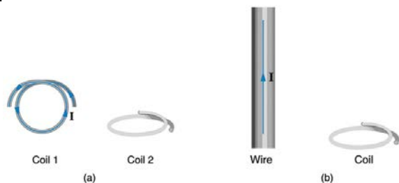
Figure 23.56 (a) The planes of the two coils are perpendicular. (b) The wire is perpendicular to the plane of the coil.
